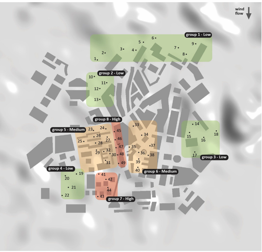
Location of test probes and their groups marked on the model with natural terrain and buildings. The probe locations and number are the same for both Case A and Case B. 49 representative locations, divided into seven groups, were selected within the built area for test probes located 2m above ground.
